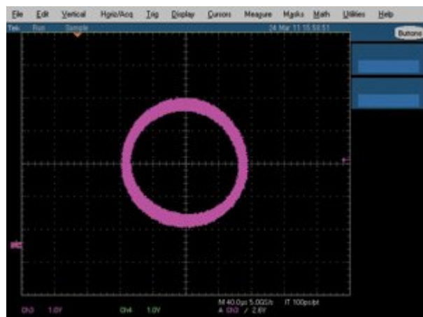
Figure 3 When swept in frequency, the phase varies from -89 to -91°.
