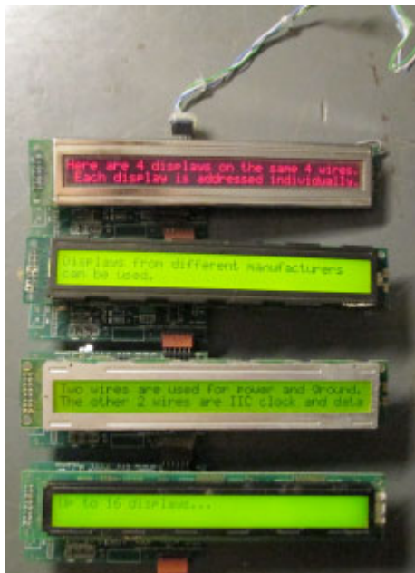
Figure 10 With each board set at a different address, I could send each display an individual and unique message. Note the different qualities and contrasts between different manufacturers. This is why you need to see a display before committing to it in a production design. Note, with the pass through wiring, each board plugs into each other board. No additional cables are needed.
