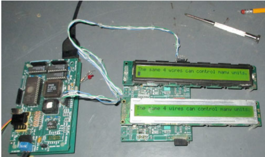
Figure 9 With both LCDs set to the same address, they both responded to a single command/data sequence and updated simultaneously.
