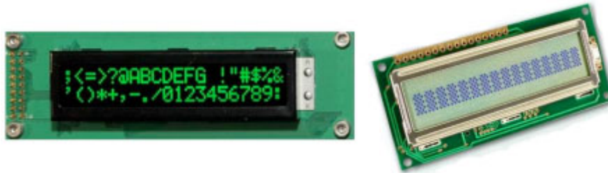
Figure 1 Although the data and control signals are the same, the two pseudo standard parallel interface styles for character displays are in a DIN style (left) or SIP style (right).
