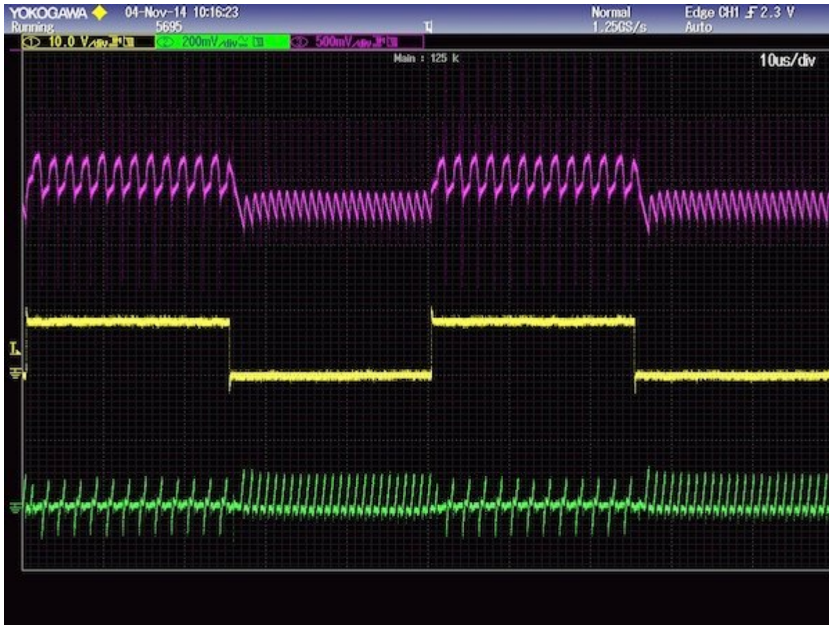
Figure 2 The top trace (pink) is the output voltage response while the middle trace (yellow) is the load current and the bottom trace (green) is the inductor current. Note the high frequency spikes have not been filtered in order to provide the unaltered response of the controller.
