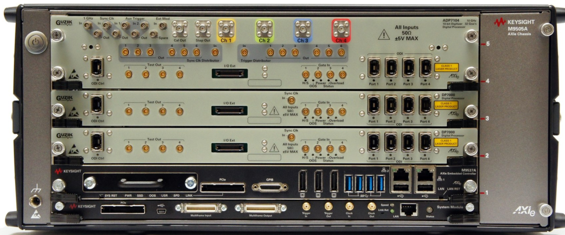
Figure 4. Guzik is the first company to announce a test product with an ODI interface. The AXIe module has four ODI ports for data and one for control signals.
